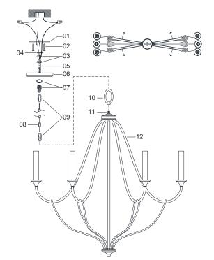
Components 01. Mounting Bar w/Green Screw 02. Outlet Box Mounting Screws 03. Hex Nuts 04. Washer 05. Nipple 06. Canopy 07. Threaded Ring & Screw Collar Loop (1/8-27IP) 08. Chain 09. Chain Links 10. Loop 11. Fixture 12. Arm
